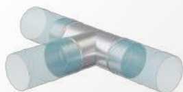
Tees for round air ducts of different diameters
